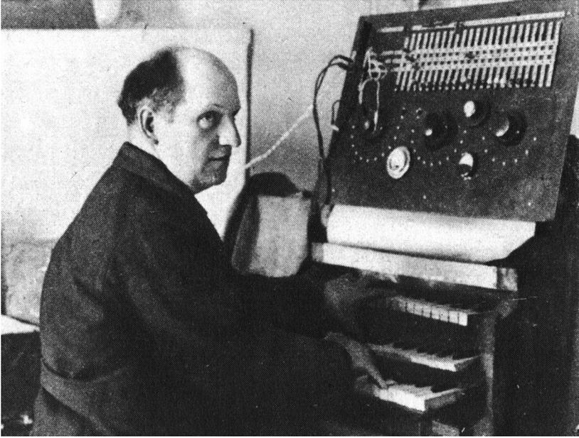
**FIGURE 13.** Jörg Mager playing the three-manual Partiturophon, circa 1930. Note how his left hand is fingering keys on both the upper and the middle manual: this technique was required for polyphonic playing, as each manual could sound only one tone at a time. Source: Andy Mackay, *Electronic Music* (Minneapolis: Control Data Publishing, 1981), 19.
