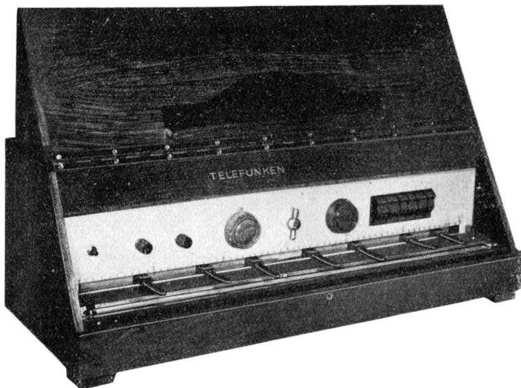
**FIGURE 23.** The Telefunken-Trautonium, also known as the Volkstrautonium.
